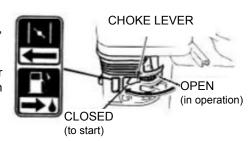
The "CLOSED" position of the choke lever enriches the fuel-air mixture. This is required to start (at cold start as well as a warm start) of the engine. The "OPEN" position provides the correct fuel-air mixture to the engine during normal work (after the start) available.
